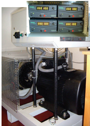
Custom built 50kW motor loading jig
