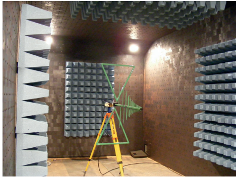
Fully lined anechoic chamber and radiated emission antennas
