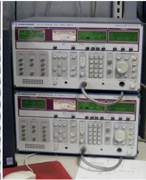
Rhode and Schwarz EMC test receivers covering conducted and radiated emission frequency ranges from 9kHz to 3.6GHz
