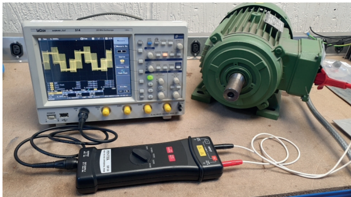
Oscilloscope and high voltage differential probe used to measure waveform characteristics at motor terminals
